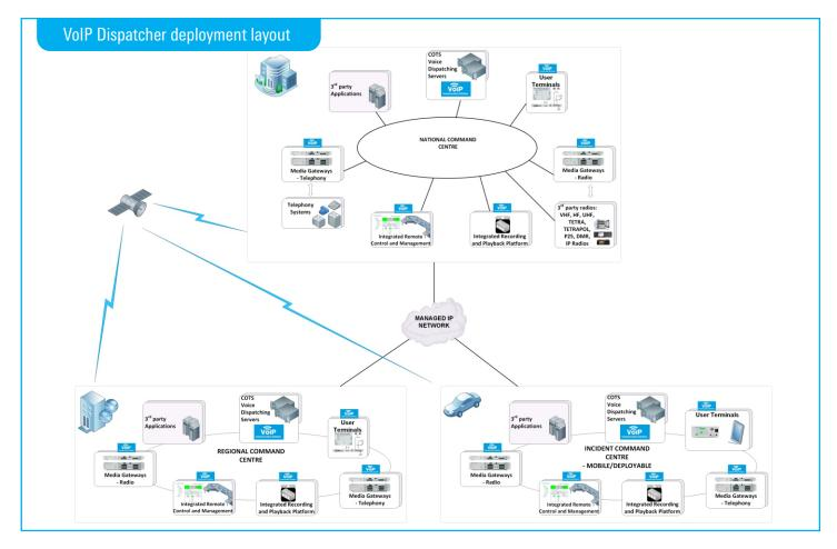
The VoIP Dispatcher is adaptable to the end-user specific operational and technical views, mapping the command structure layouts from one to many users (virtual unlimited capacity) and under different servers and network topologies, inclusive Virtual Environment or segregated networks.
